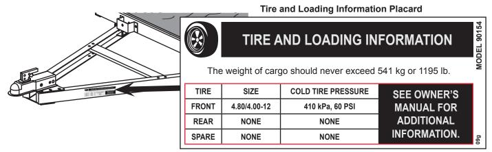
Figure Q: Tire and Loading Information Placard Location
